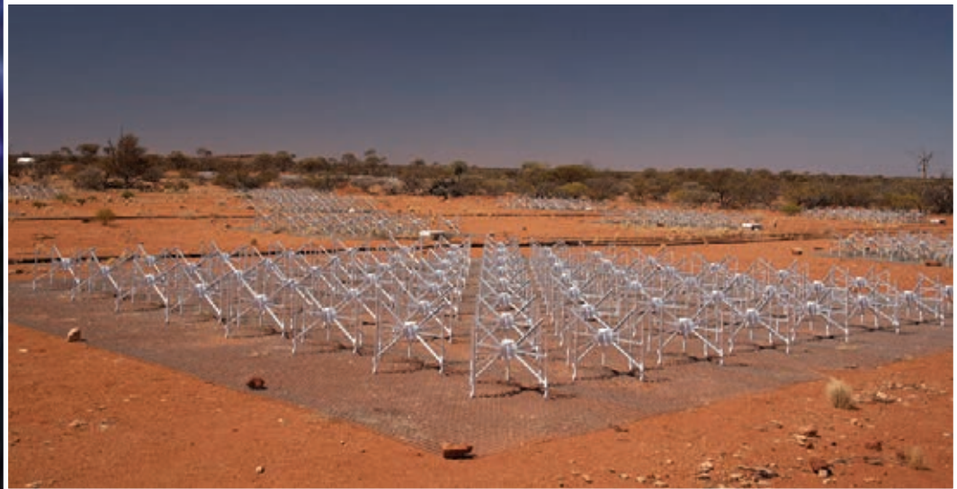
Photograph of the CRAM, a new 8x8 dipole tile sitting within the centre of the southern hexagonal subarray of the MWA.
