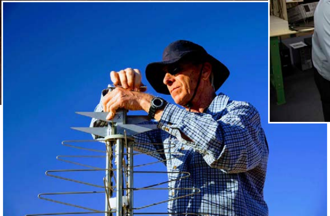
Above: SKA engineer Mark Waterson deploying the latest SKA-LOW antenna.
