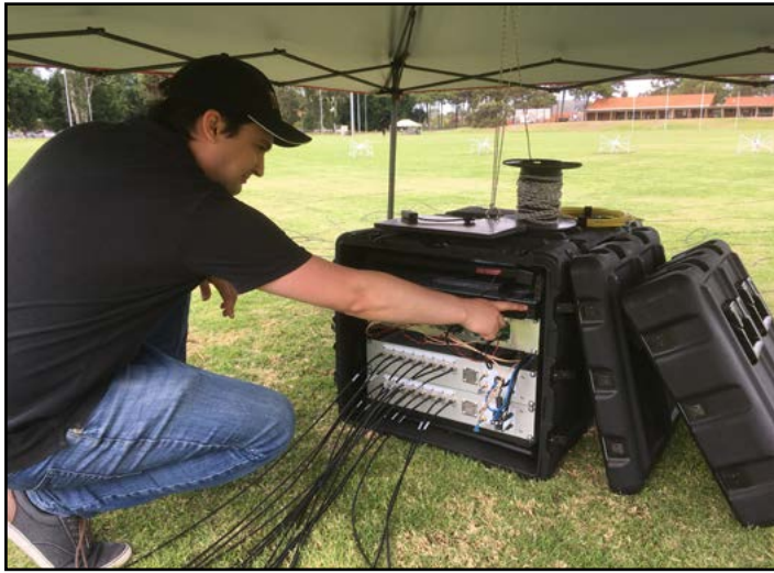
IMAGE LEFT : Engineer Jake Jones starting the SDA receivers during a deployment test on Curtin University's sports ovals. IMAGE CREDIT: Randall Wayth
