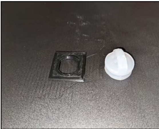
IMAGE ABOVE: Figure 12: Silicone Grommet with a test N-type connector cut-out. IMAGE CREDITS: Luke Verduyn
