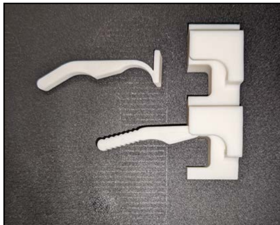
IMAGE ABOVE: Figure 3: Second RTL SDR cradle and clamp prototype. Credit: Luke Verduyn
