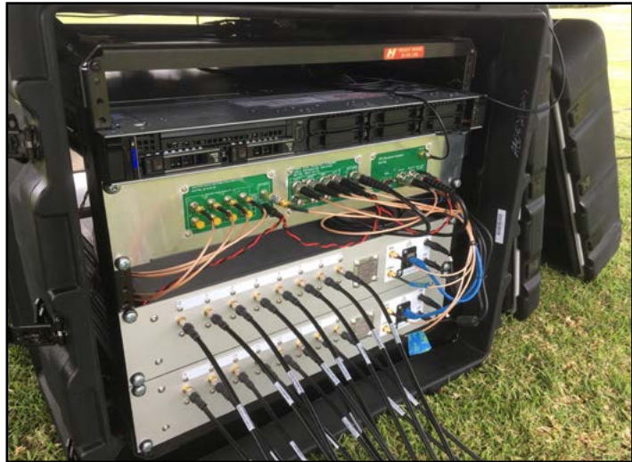
IMAGE RIGHT : The assembled receiver, clock and computing units, housed in a ruggedised container, during testing on Curtin University's sports ovals. IMAGE CREDIT: Randall Wayth
