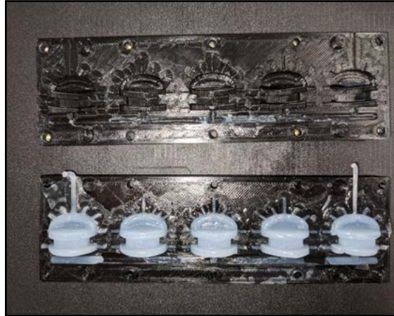
IMAGE ABOVE: Figure 11: Filled mould. IMAGE CREDITS: Luke Verduyn
