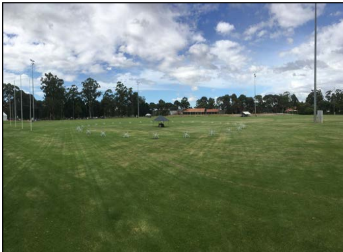
IMAGE LEFT: The system deployed on Curtin University sports ovals, with 32 MWA dipole antennas in a 35 metre diameter ring. IMAGE CREDIT: Randall Wayth
