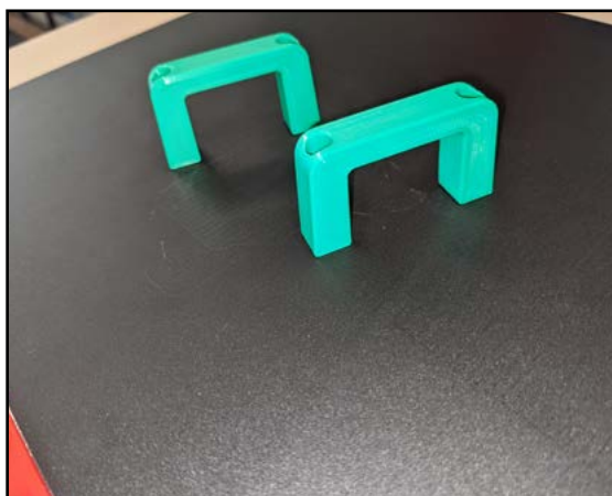
IMAGE ABOVE: Figure 8: USB port clamps. IMAGE CREDITS: Luke Verduyn
