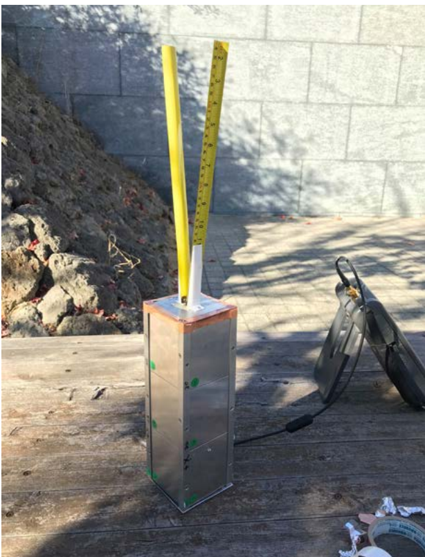
Figure 1 3U CubeSat tri-band antenna prototype for ionospheric measurement.
