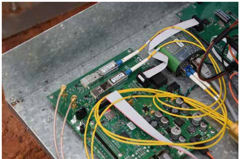
A close-up view of the ASTRON RFoF modules, connected to optical fibre and USB inputs of the beamformer interface (BFIF) board. Image Credit: Curtin University.
