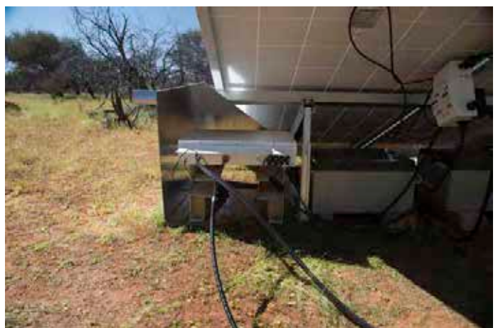
The long baseline tile controller containing monitor and control equipment, sitting in place underneath the solar panels of a deployed tile. Image Credit: Curtin University.
