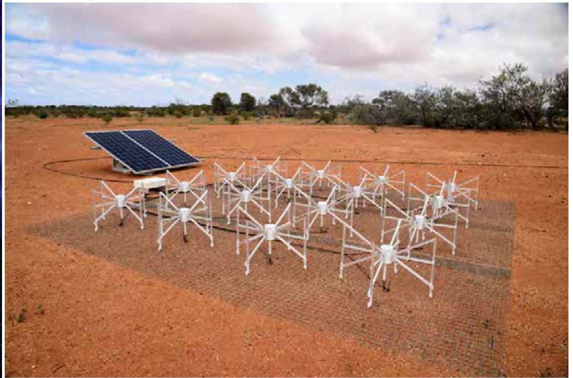
A complete long baseline tile, September 2017. Image Credit: Kim Steele, Curtin University
