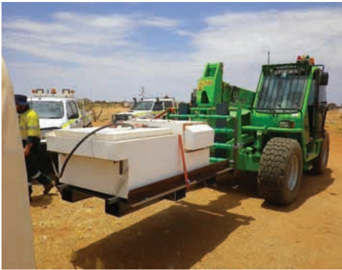
Figure 3, above: A MWA receiver (white box) secured to the new lifting frame on an all-terrain telehandler, to be installed at a new location. Credit: Curtin, 2019
