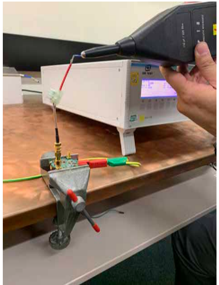
Figure 3, above: Laboratory electrostatic discharge test. Credit: Kovaleva, 2019
