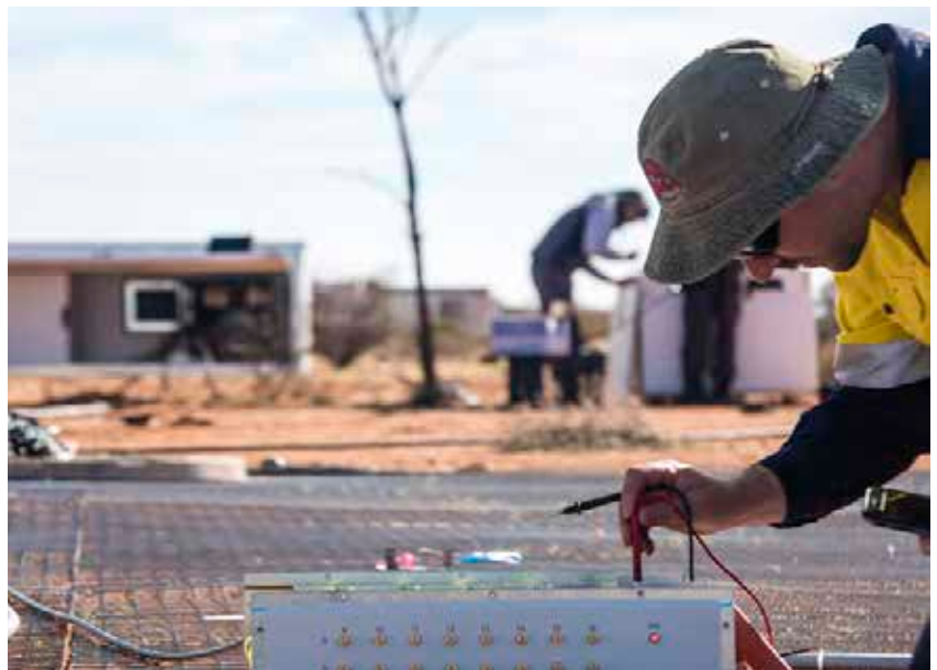
Figure 8, right: Balance contractor testing the electrical connections on a SMART box. Credit: ICRAR, 2019
