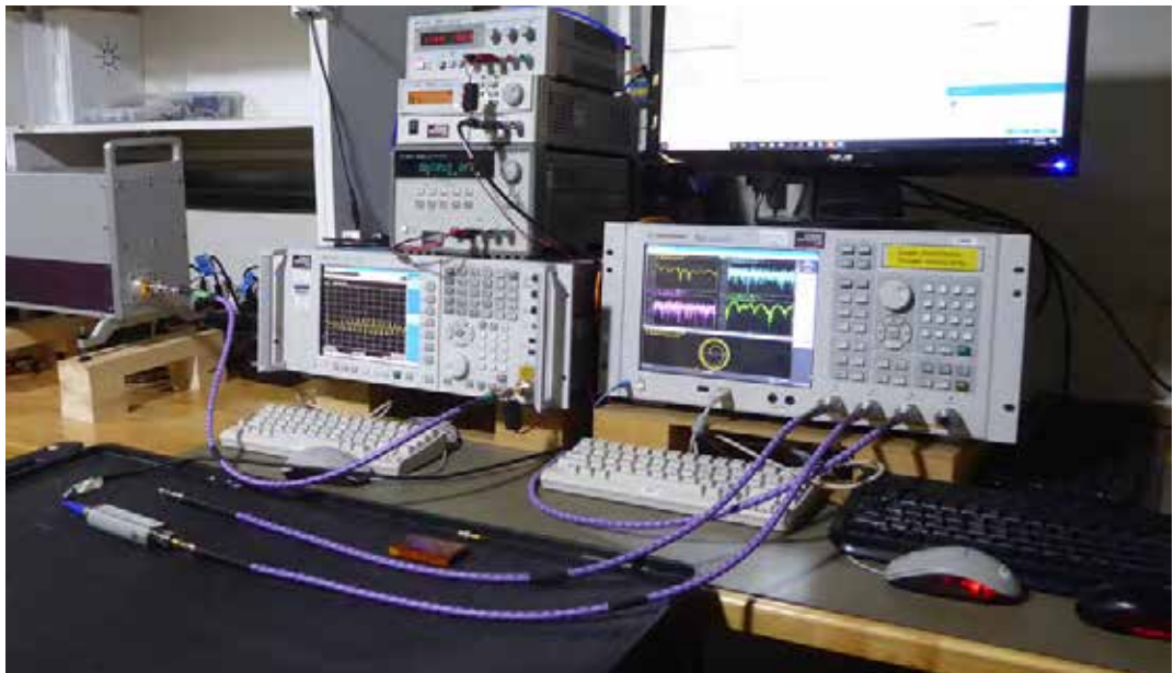
Figure 1, above: Noise parameter extraction setup in the CIRA lab.
