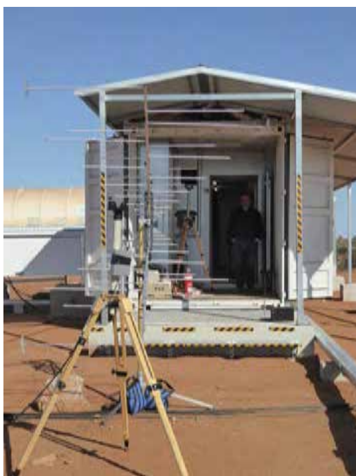
Figure 3, left: Radiated emissions testing of the FPF using high gain wideband antenna. Credit: Kenney, 2019
