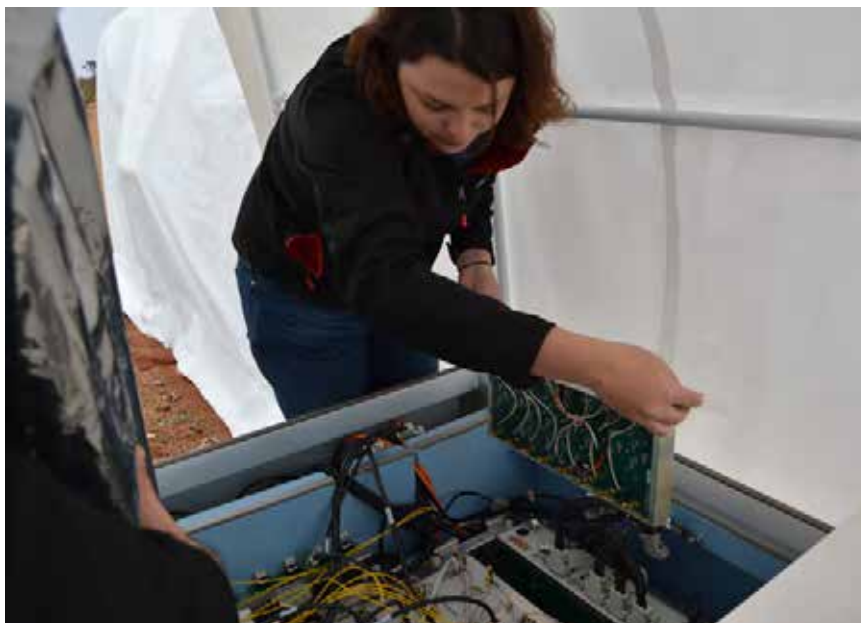
Figure 2, left: Mia Walker removing an ASC module from inside a receiver on site. Credit: Curtin
