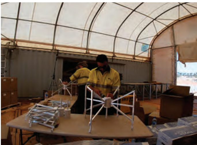
Figure 5, above: Geraldton contractors building MWA dipole antennas for EDA2. Credit: Curtin, 2019
