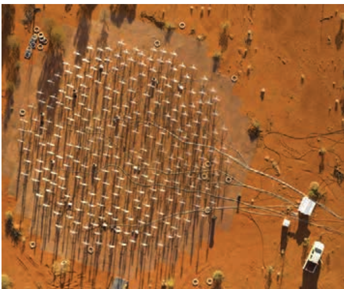
Figure 5, above: Phase 2 from above, showing the complete AAVS2 array with 256 antennas deployed and connected to SMART boxes, and the FNDH to the right. Credit: ICRAR, 2019
