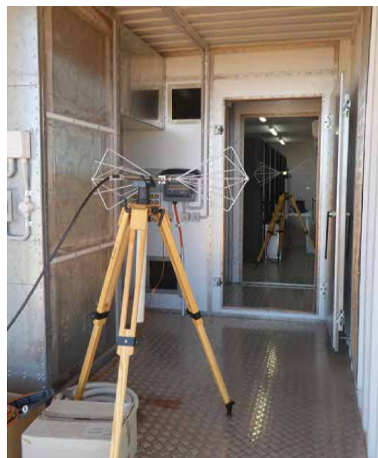
Figure 3, left: Radiated emissions testing of the FPF using high gain wideband antenna. Credit: Kenney, 2019
