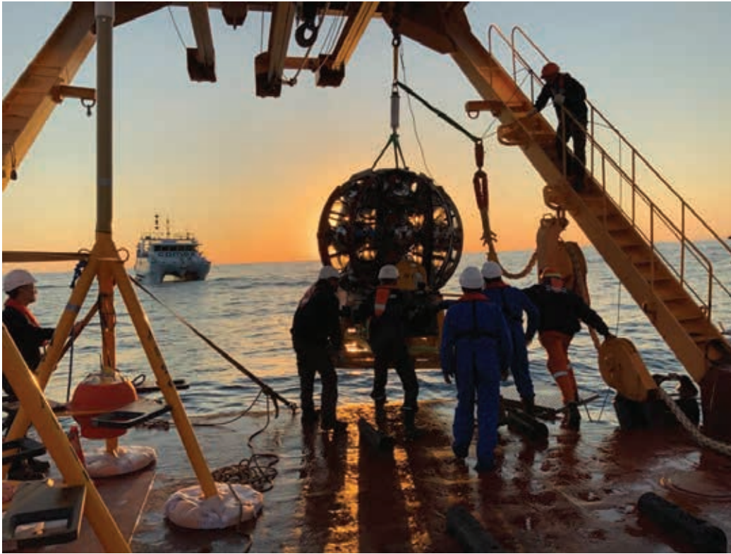
Figure 1, left: A KM3NeT detection unit prior to deployment. Below: the unit on the sea floor, awaiting an acoustic signal to unravel. Credit: KM3NeT Collaboration
