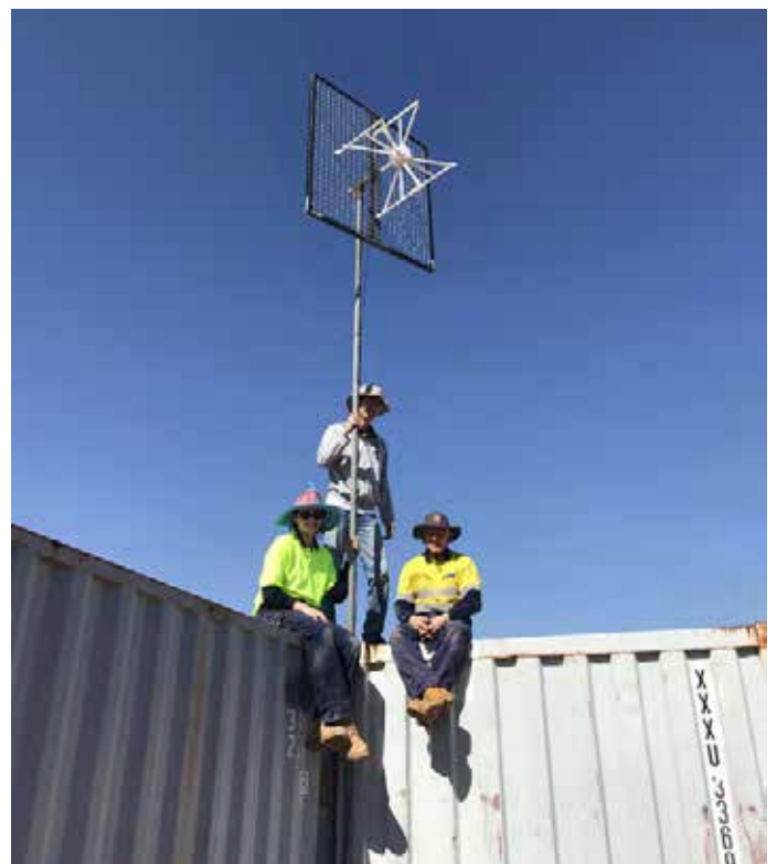
Figure 9, above: The 'dipole on a pole' deployed at site to detect radio interference from Geraldton. Credit: Curtin, 2019
