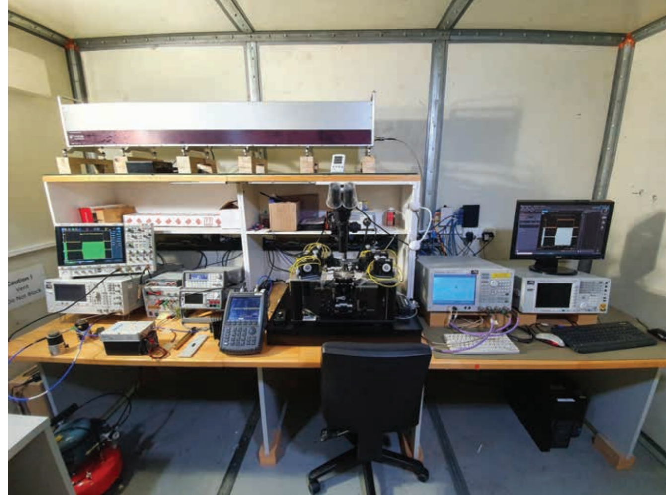
Right: The measurement set-up for HPM injection and semiconductor characterisation at the CIRA laboratory. Credit: Silvestri
