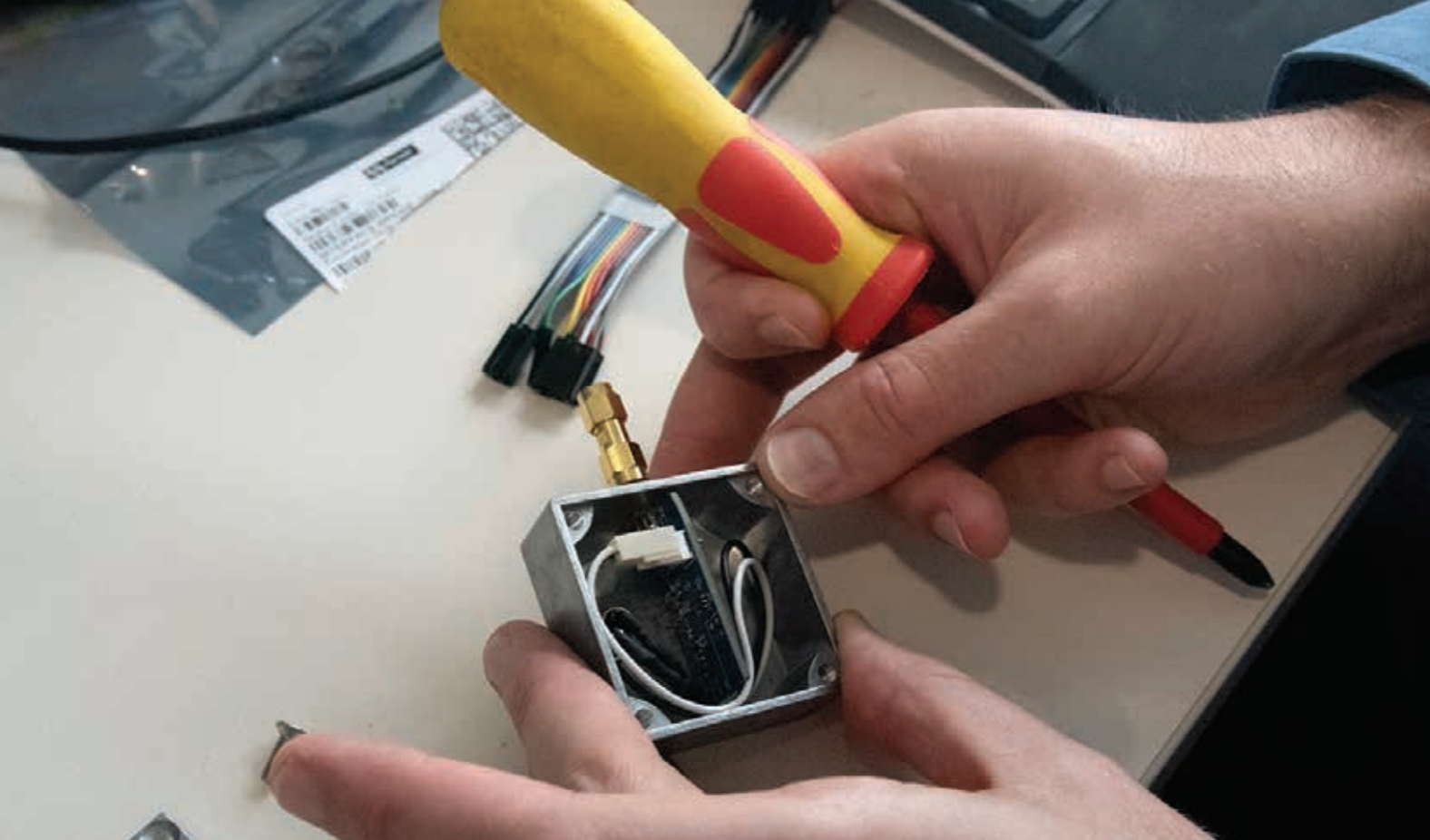
Above: Opening up the test jig for a low-noise amplifier. Credit: Curtin
